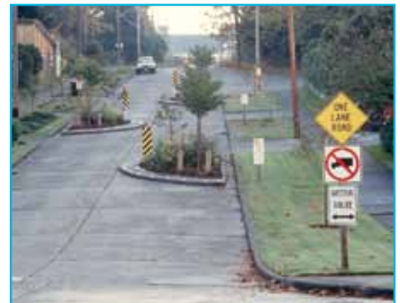
Midblock chicanes or ‘neckdowns’ are one option to force traffic to slow down. Photo: Richard Drdul.
