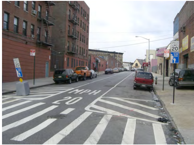
Figure 1. Typical Gateway Signage and Buffering, Claremont Neighborhood Slow Zone
